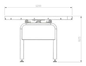
Rotary table to facilitate collection after exiting the breading machine or the frying line.
